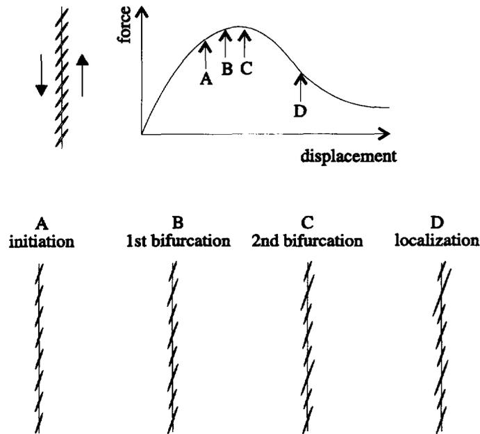
Fig. 1. Crack growth pattern observed in torsion shear experiment.
