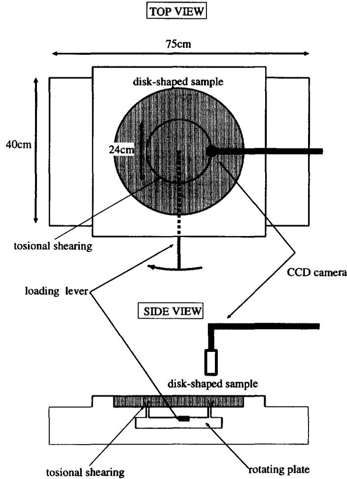
Fig. A1. Equipment for torsion experiment.
