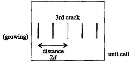
↑ effect of growing 1st crack on 3rd crack can be evaluated by using Green function of infinite body
