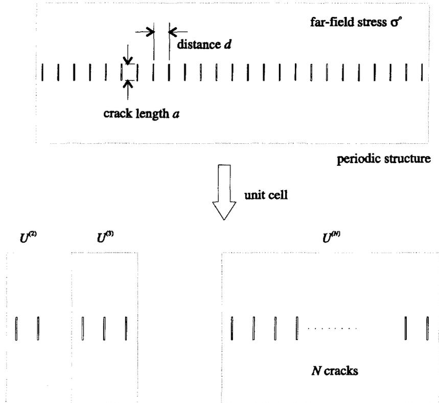
Fig. 2. Periodic structure of cracks.
