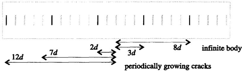
Fig. 3. Evaluation of interaction in unit cell using periodic structure.
